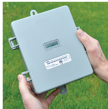
A load control receiver.
